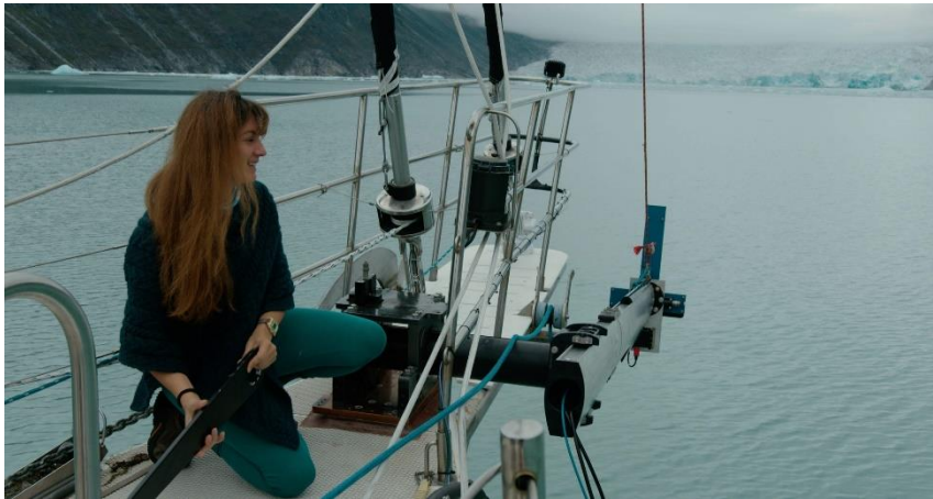
Figure 2 Pole-mounted Multibeam Echosounder 2022 - Greenland
