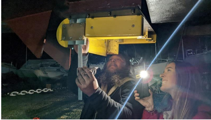
Figure 3 multibeam sonar hull installation in the yard
