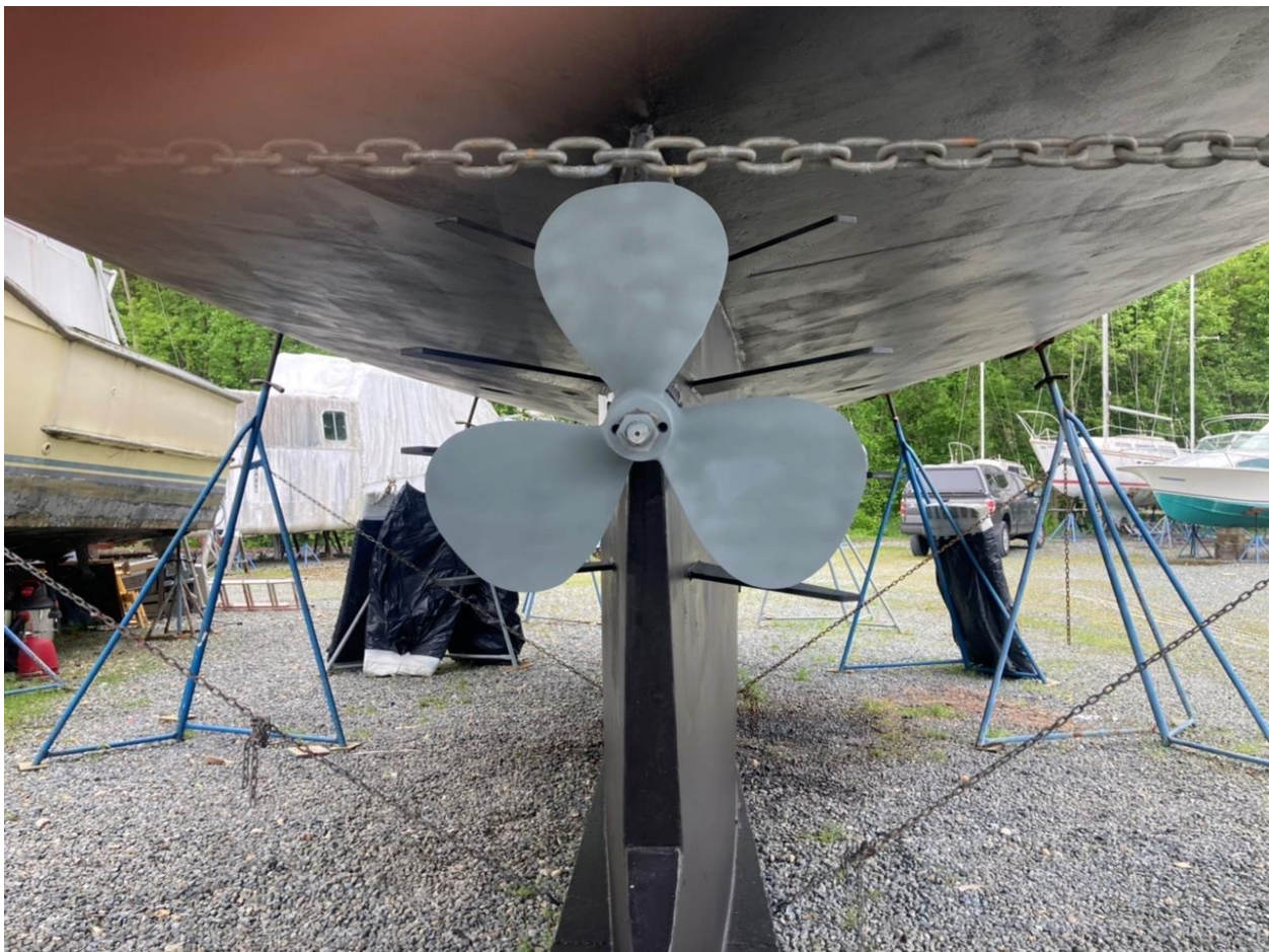
Figure 4 Propeller Installation and welded Ice-deflectors
